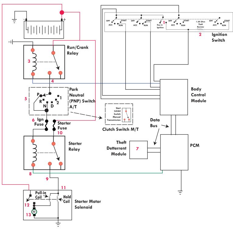
1). Key is inserted into lock cylinder and signals BCM (1).
