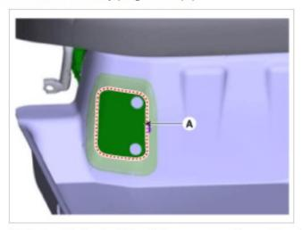
3. Unfasten the hook (A) and then remove the safety plug (C) by pulling the lever (B) to the direction of arrow.
