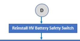
NOTE: Ignition ON and connect GDS with VCI to vehicle to perform STUI Auto VIN, then turn off vehicle ignition.
