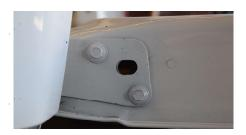
3. Loosen but DO NOT remove the lower bolt with the 10mm wrench.
