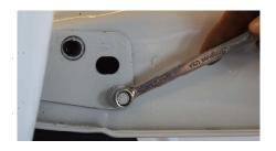
5. Apply the included thread-locking fluid to the threads of the bolt. Thread the bolt through the bottom mount plate. Tighten the loosened lower bolt with a 10mm wrench.
