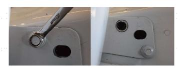
4. The bottom mount plate has a slot in one of its corners. Position the plate between the washer of the loosened lower bolt and the tailgate with the loosened tailgate bolt in the slot of the mount plate.
