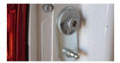
8. The included mylar sheet can prevent components from rubbing against the truck bed and tailgate in the event that parts become loose. Cut the mylar sheet to the required size with a pair of scissors. Apply the mylar sheet to the truck bed and tailgate where tailgate assist components come close to contact during operation.
