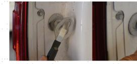
7. Insert the previously removed cable bolt through the hole of the top mount plate and reinstall the cable bolt with the mount plate onto the vehicle with the included torx wrench or a T50 torx socket.
