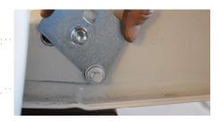
6. Remove the tailgate cable from the cable bolt, and then use the included torx wrench or a T50 torx socket to remove the cable bolt.
